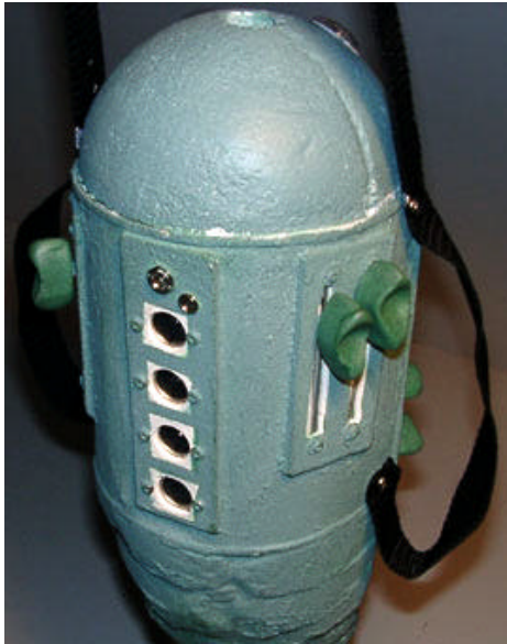
Photo 3: Close up of MIDI, power and MIC sockets
