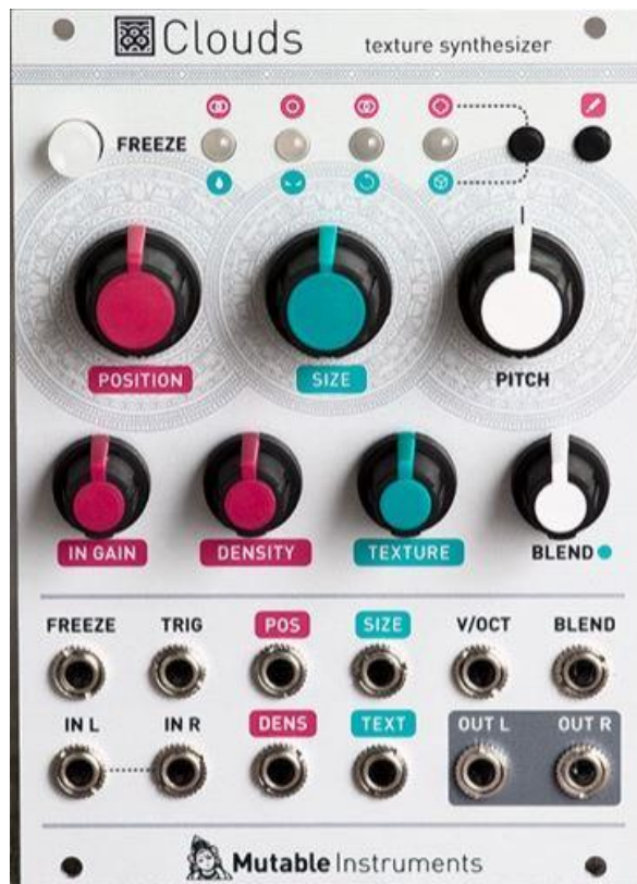
Figure 5: The physical interface for the Clouds texture synthesizer.
