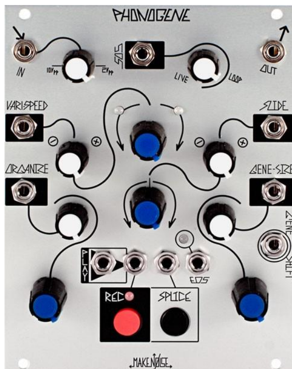
Figure 4: The physical interface for the Phonogene.
